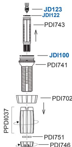
7. Push complete injection stem assembly in position at the bottom of the blue body, making sure desired scale is facing front of injector. Keys at the top of the black sleeve should slide into the slots at the bottom of the body. Slide injection stem nut (PDI702) up the sleeve and screw back on. Insert hose back onto the bottom of the check valve barb (PJDI118). Screw hose nut (PDI748) back on.
